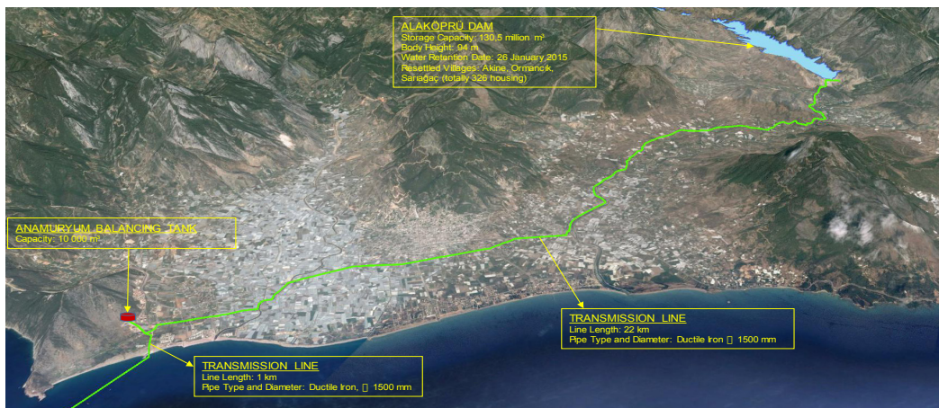
Figure 4: Pipeline and balancing tank
