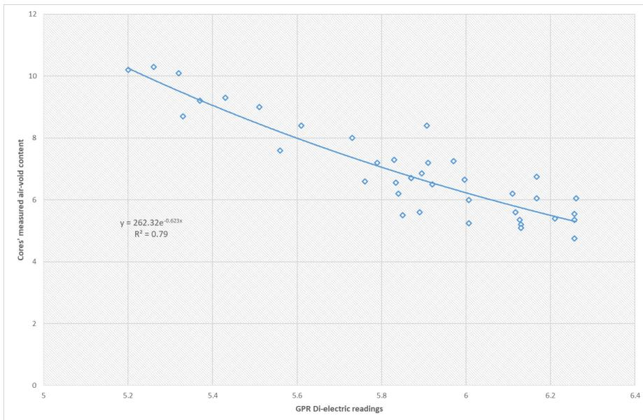
Figure 3: Relationship between GPR di-electric readings and air voids content of extracted cores
