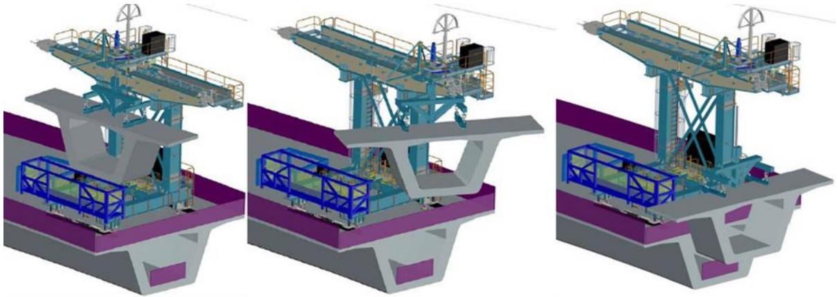
**Fig. 6:** Installation of Precast concrete Segments using Lifting Frame
