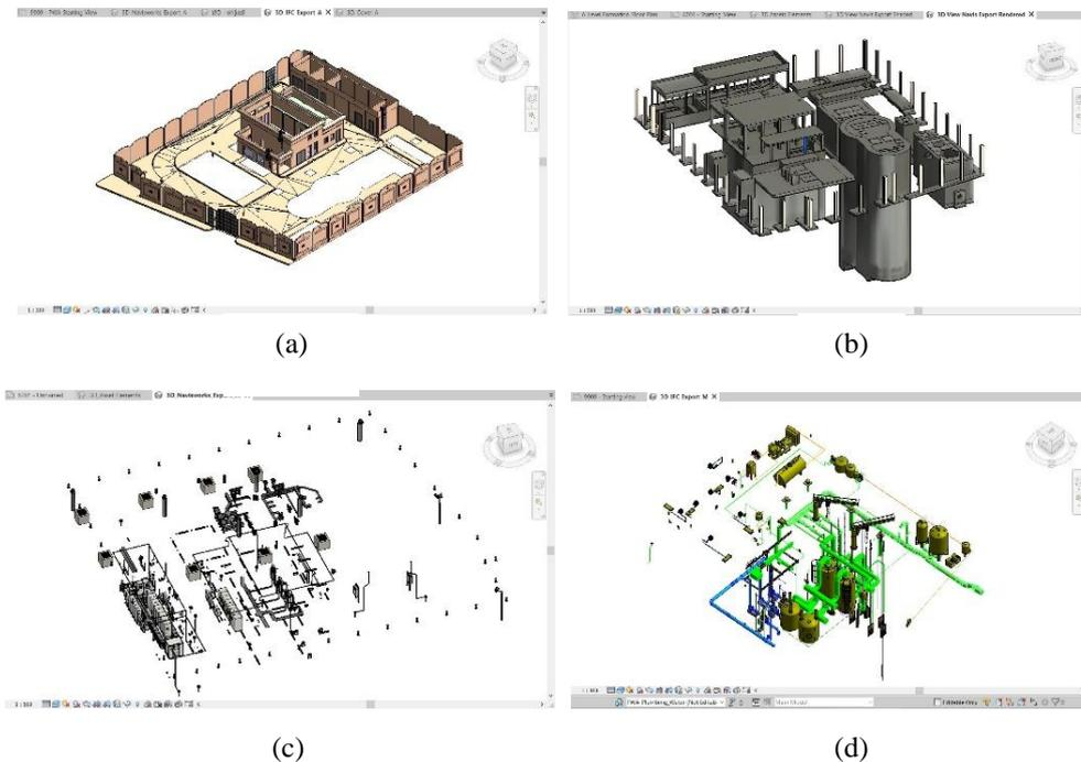
**Fig. 1** BIM Model Files: (a) Architecture Model (b) Structural Model (c) Mechanical Model (D) Electrical Model
