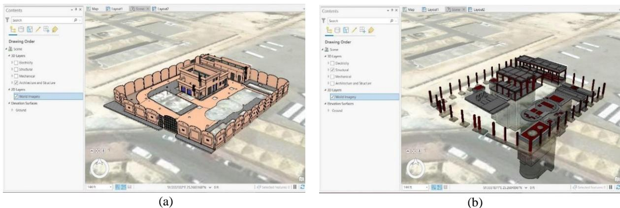
**Fig. 4:** Pumping Station Project PS16 North/PS16: (a) 3D GIS Architecture Model (b) 3D GIS Structure Model
