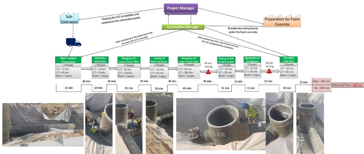
Fig. 1: Current State of Manhole’s Connection Process
