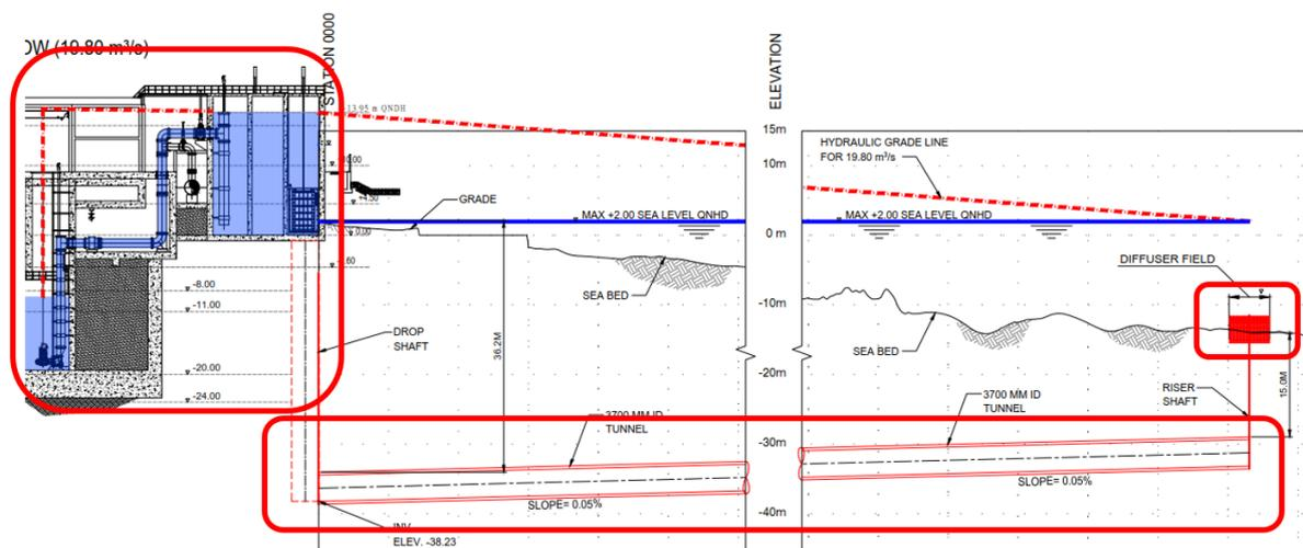
Fig. 2: Gravity flow system
