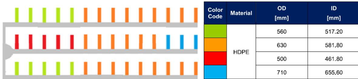
Fig. 5: Diffuser field piping arrangement and size
