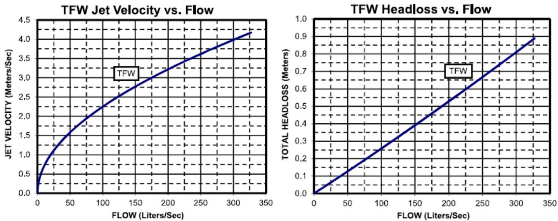
Fig. 3: Duckbill valve charts - Jet velocity vs Flow Rate and Head loss vs Flow Rate (courtesy of Tidelfex)
