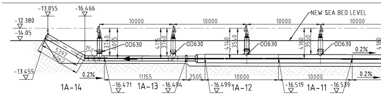
Fig. 6: Longitudinal section of diffuser pipes and ports
