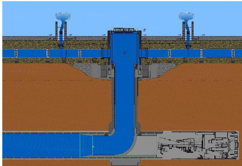
**Fig. 8:** Final stage of diffuser field section-Operational phase
