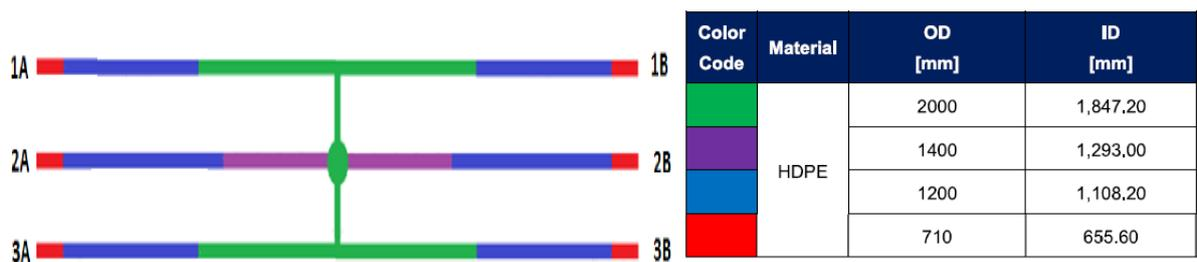
Fig. 4: Diffuser field piping arrangement and size
