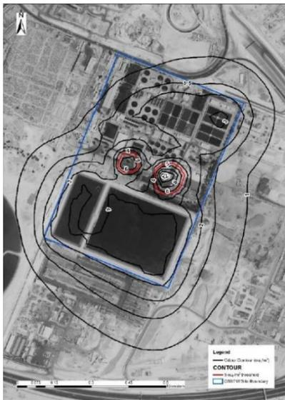
**Fig. 6:** Contour Plot of Scenario 3 Maximum 98<sup>th</sup> Percentile Odour Impacts (ouE/m<sup>3</sup>)
