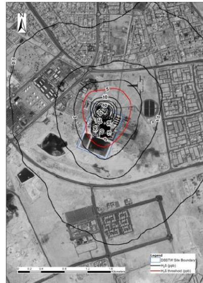
**Fig. 5:** Contour Plot of Scenario 2 Maximum 98<sup>th</sup> Percentile H<sub>2</sub>S Impacts (ppbv)
