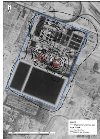
**Fig. 7:** Contour Plot of Scenario 3 Maximum 98<sup>th</sup> Percentile H<sub>2</sub>S Impacts (ppbv)
