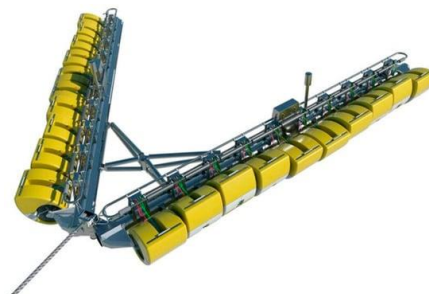
Fig. 3: WEPTOS WEC structure
