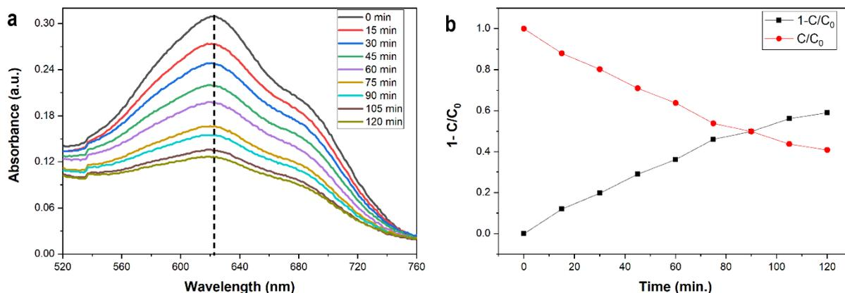
**Fig. 3:** a) DG23 dye degradation and b) time span vs  $1-C/C_0$  for the DG23 dye decolorization over Tb<sup>3+</sup> doped La<sub>10</sub>Si<sub>6</sub>O<sub>27</sub> UV photo catalyst
