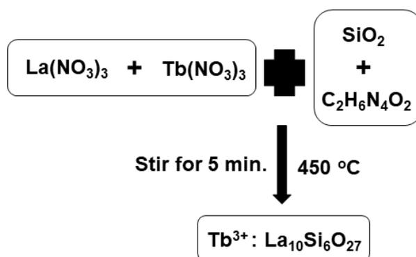
**Fig. 2:** Synthesis procedure of  $\text{Tb}^{3+}$  doped  $\text{La}_{10}\text{Si}_6\text{O}_{27}$  material
