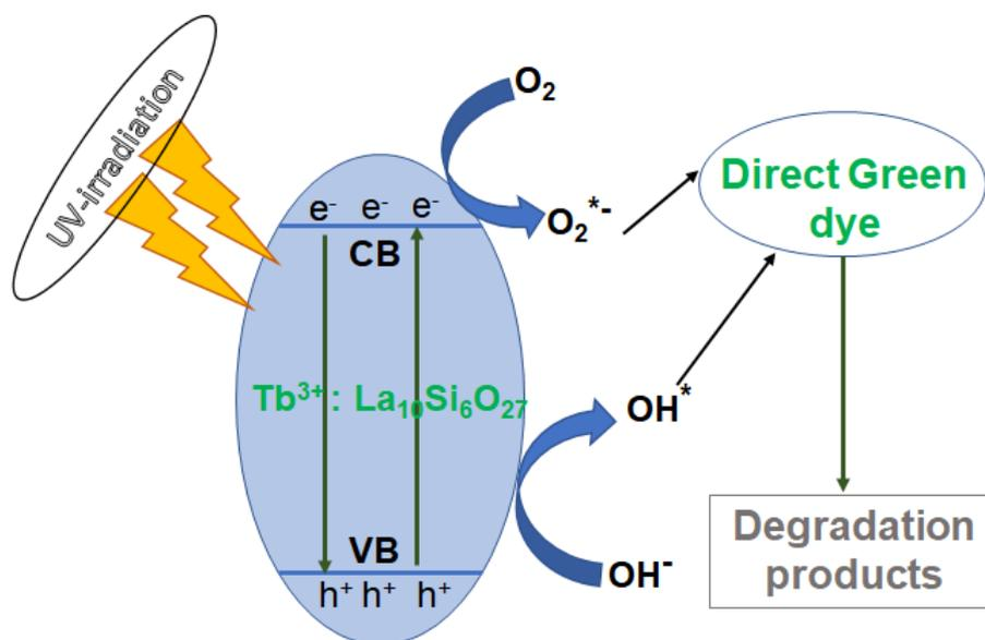
**Fig. 4:** Mechanism of DG23 dye degradation over 5 mol%  $\text{Tb}^{3+}$  doped  $\text{La}_{10}\text{Si}_6\text{O}_{27}$  photocatalytic activity under UV light illumination
