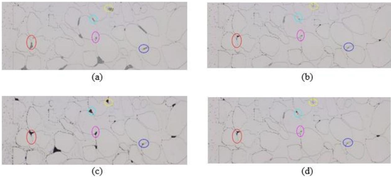
**Fig. 2:** Residual gas bubbles blocking colloid attachment and pore clogging prior to dissolving. Images (a) through (d) are ordered chronologically, with (a) being acquired first, and (d) being acquired last
