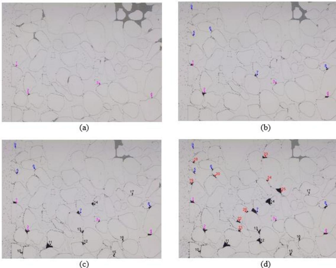
**Fig. 1:** Accumulative clogging through developing pathways. (a) was acquired at 10:46, (b) was acquired at 10:51, (c) was acquired at 10:53, and (d) was acquired at 10:54. The colors indicate when each clogging event occurred. The colours of purple, blue, black, and red indicate clogging developments for images (a) through (d) chronologically, respectively.
