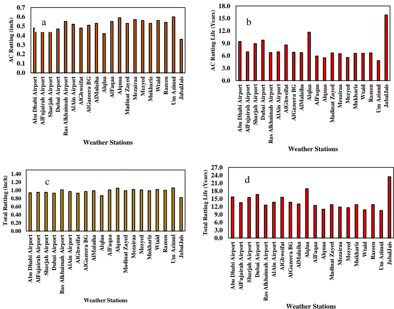
Fig. 4: Simulated (a) AC Rutting; (b) AC Rutting Life; (c) Total Rutting; and (d) Total Rutting Life for Different Weather Stations
