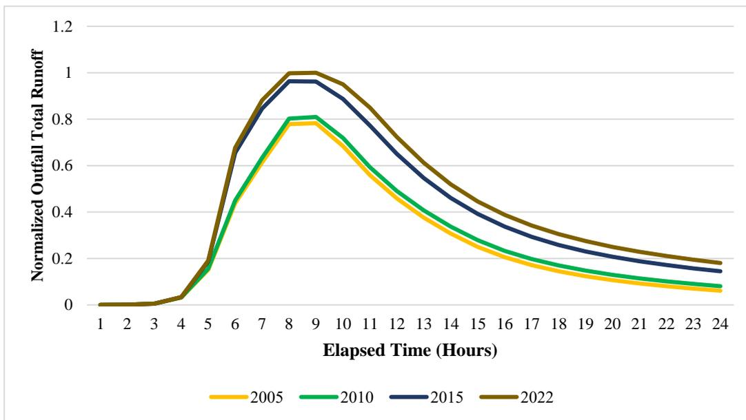
**Fig. 6:** The peak flow generated for different LULC scenarios
