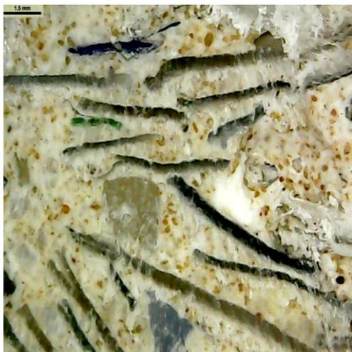
**Fig. 10:** Mortar based gypsum + 25% of PET particles
