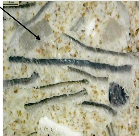
**Fig. 9:** Mortar based gypsum + 20% of PET particles
