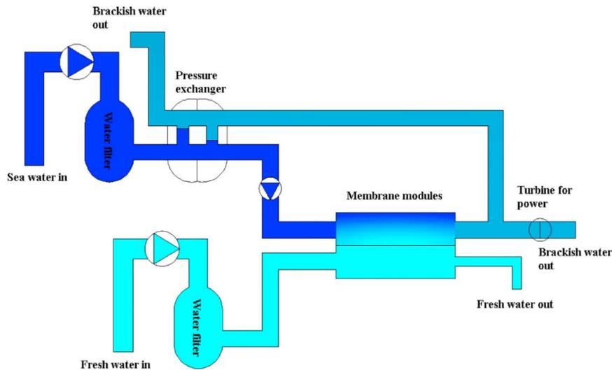
**Fig. 4:** Process outline for a standard osmotic power plant
