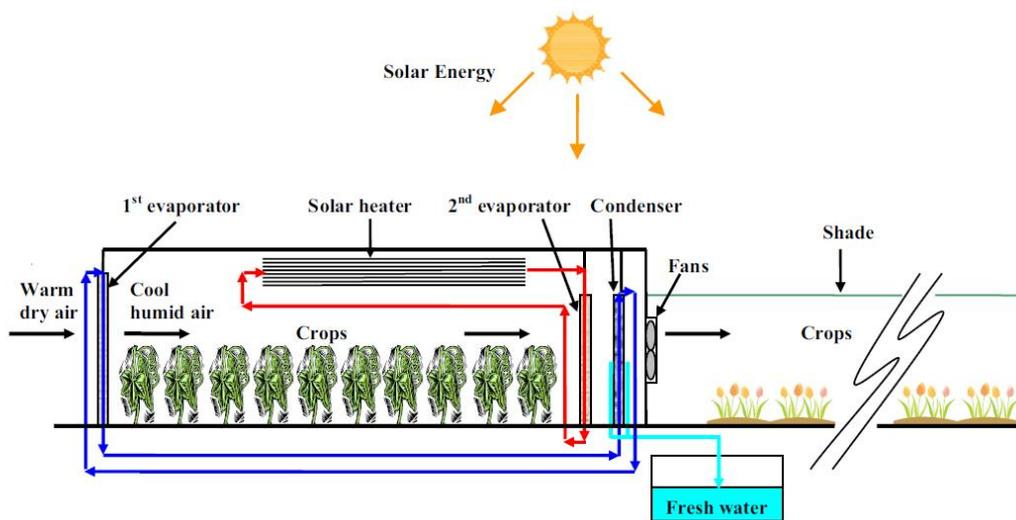
**Fig. 3:** Diagrammatic representation of the seawater greenhouse system in Oman
