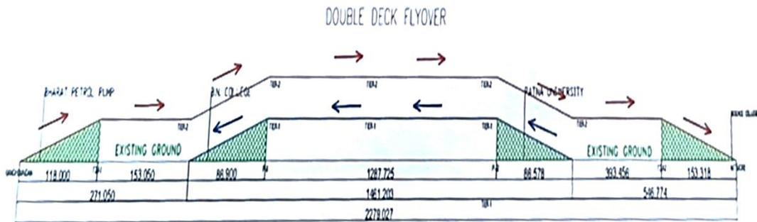
**Fig. 3:** Sectional Elevation of Double decker flyover on Ashok Rajpath
