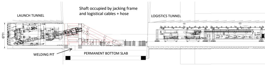
**Fig. 8: TBM Pre-assembling works through shaft**
