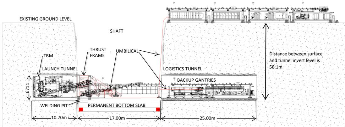
**Fig. 6: TBM Umbilical launch Illustrative sketch**
