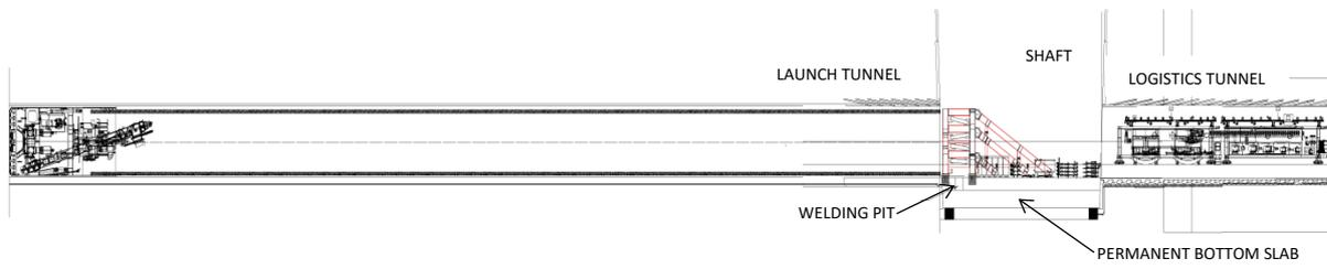
**Fig. 9:** TBM mining through umbilical system
