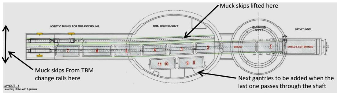
**Fig. 4:** Plan view of Logistic shaft and SEM logistic tunnel
