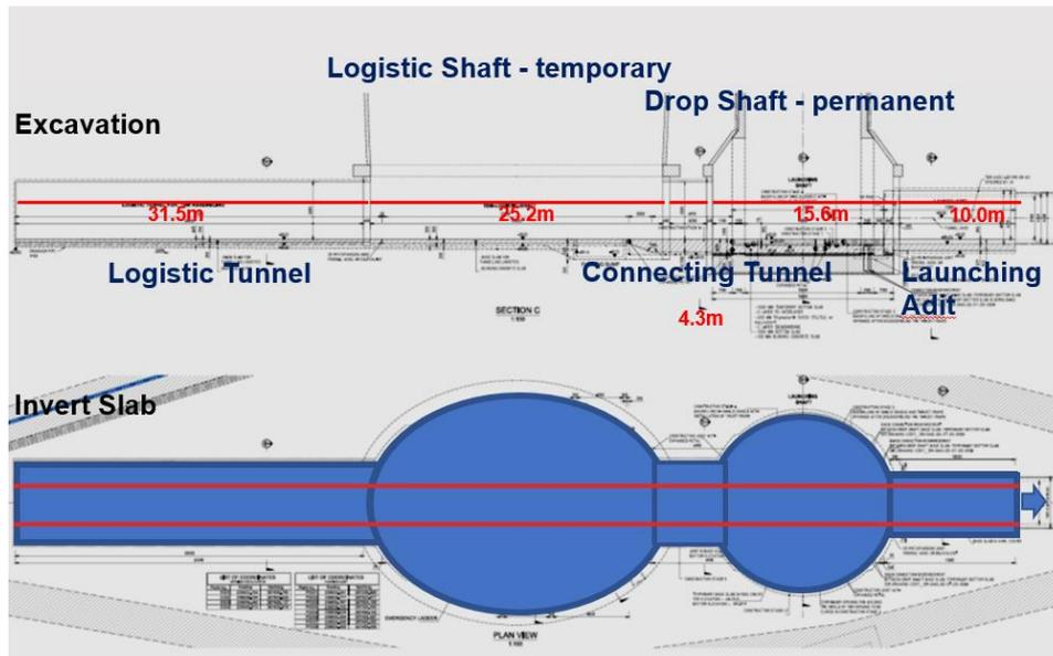
**Fig. 3:** Cross section and Plan view of Logistic shaft and SEM logistics tunnel
