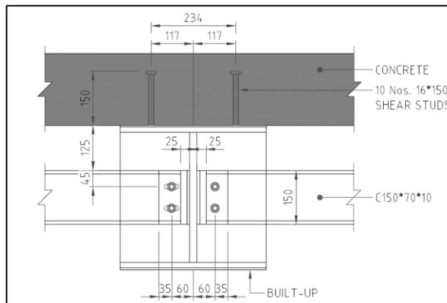
**Fig. 8: Strut & Bracket (Section) (dimensions in mm)**
