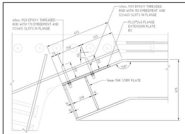
**Fig. 5:** Bracket (Section) (dimensions in mm)
