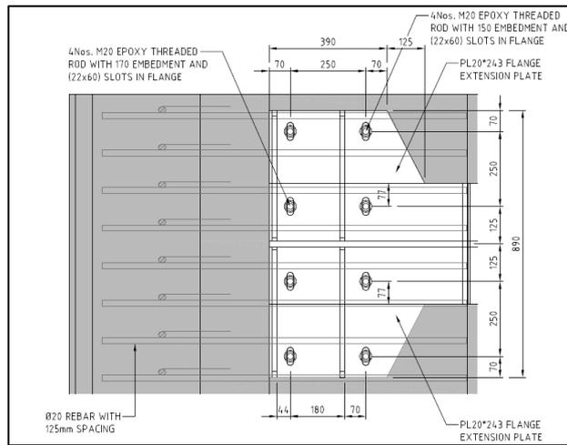
**Fig. 6: Bracket (Plan view) (dimensions in mm)**
