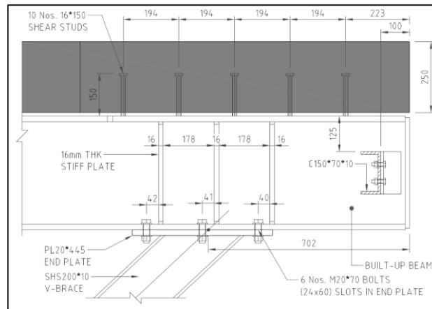
**Fig. 7: Strut & Bracket (Section) (dimensions in mm)**
