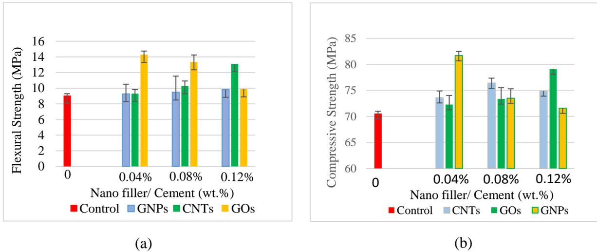
**Fig. 1:** (a) Flexural Strength Test Results, and (b) Compressive Strength Test Results
