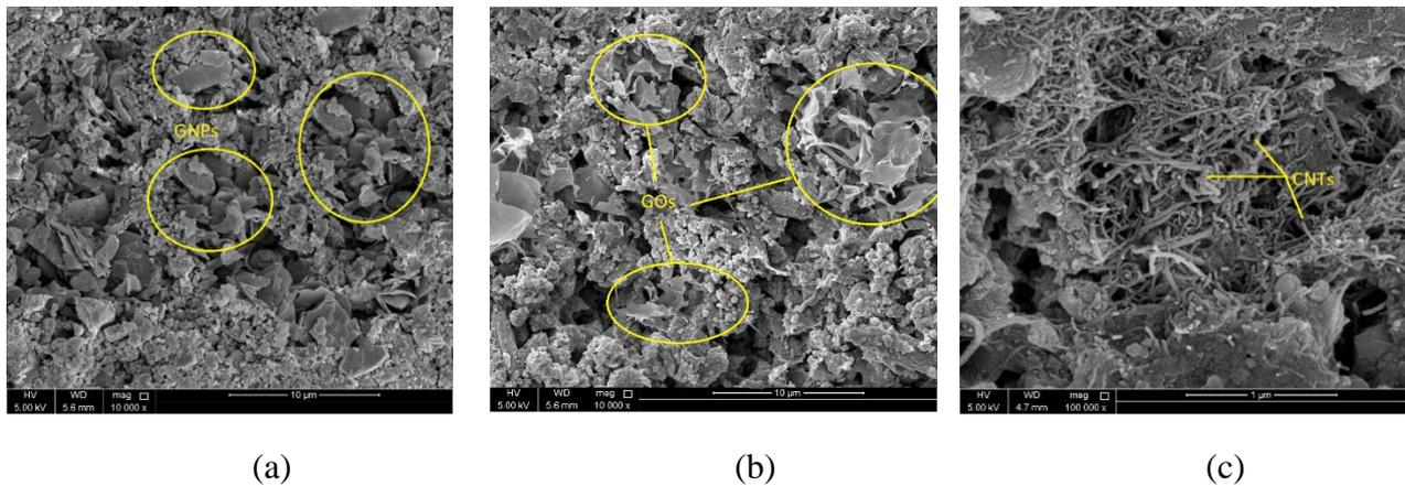
**Fig. 2:** SEM image of mix containing (a) 0.12wt. % GNPs, (b) 0.12wt. % GOs, and (c) 0.12 wt. % CNTs
