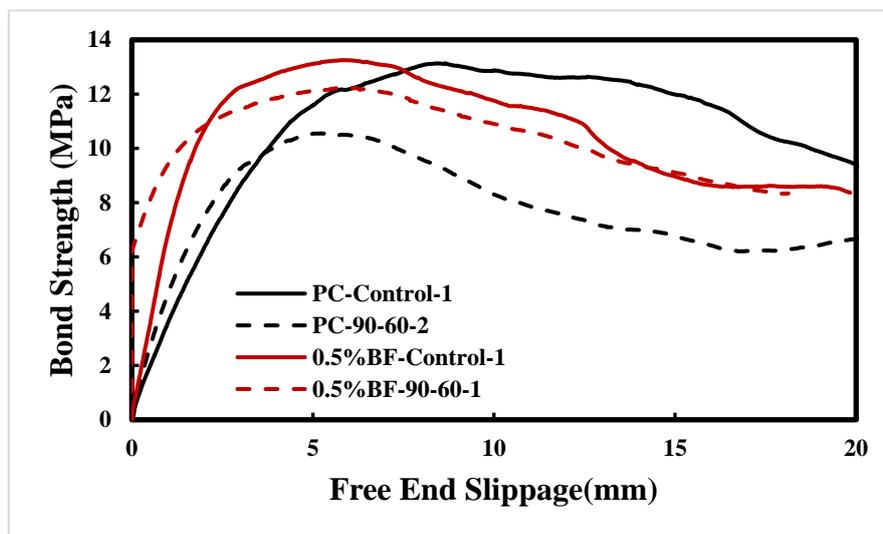
Fig. 3: BFRP Bars Bond-Slip Response
