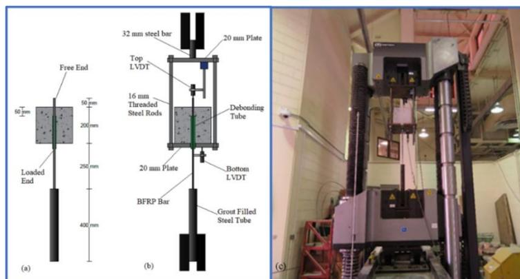
**Fig. 1:** (a) Details of Specimens for Pullout Test; (b) Details of Test Setup; (c) Test Setup Photo
