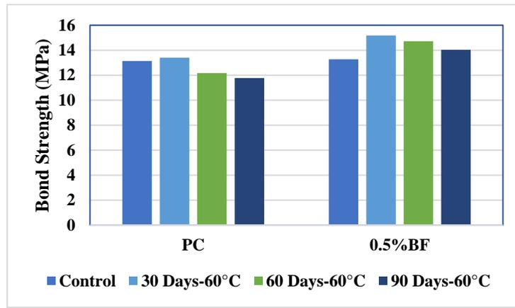
Fig. 4: Bond Degradation of HWBFRP Bars in Plain and FRC Concrete
