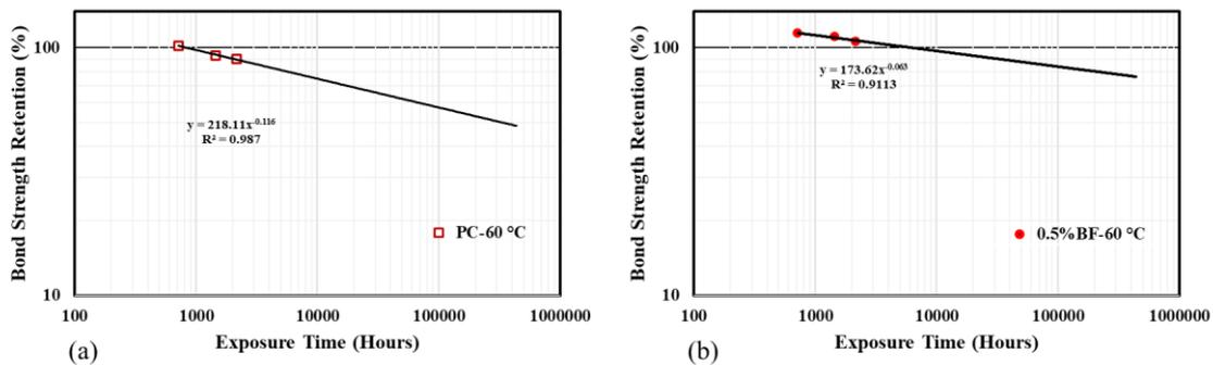
Fig. 4: Double Logarithmic Retention of HWBFRP Bars in (a) Plain Concrete; (b) FRC
