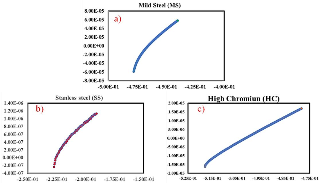
**Fig. 2:** Linear polarization resistance (LPR) curves. The slope of the LPR curve provides  $R_p$  values
