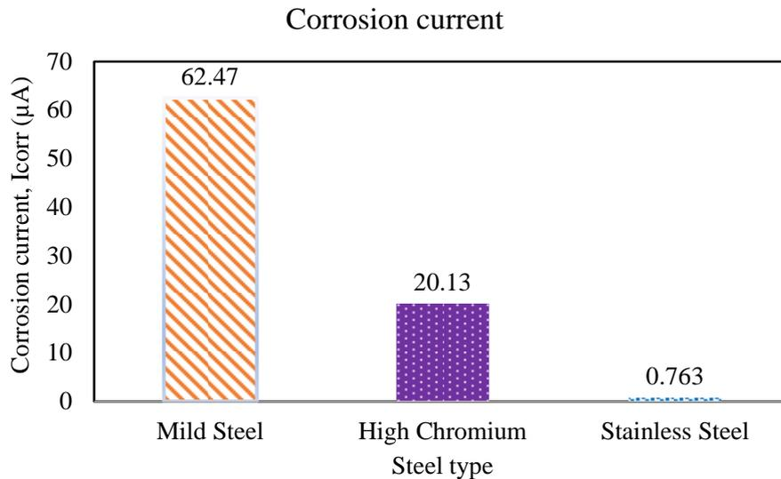
**Fig. 4:** Microcell corrosion current calculated based on the  $R_p$  values in mild steel, high chromium steel, and stainless steel
