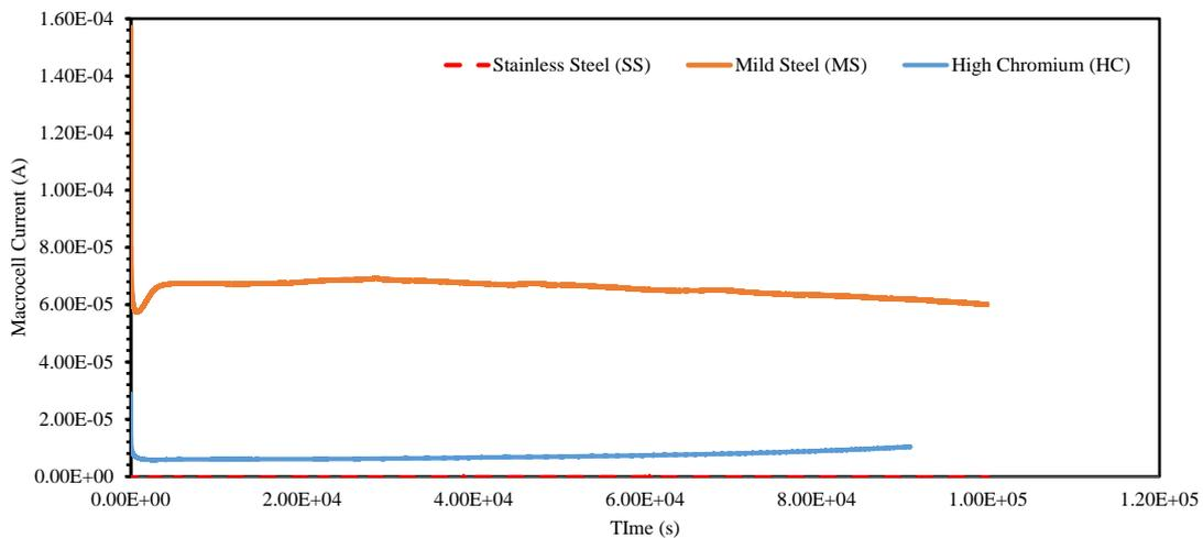
**Fig. 5:** Macrocell corrosion in block samples with an anode-to-cathode ratio of 1
