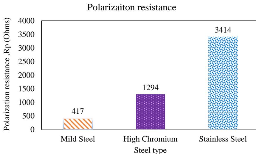
**Fig. 3:** Polarization resistance of mild steel, high chromium, and stainless steel in the active corrosion state under chloride attack
