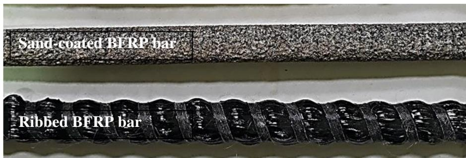
Fig. 1: The Used BFRP Bars
