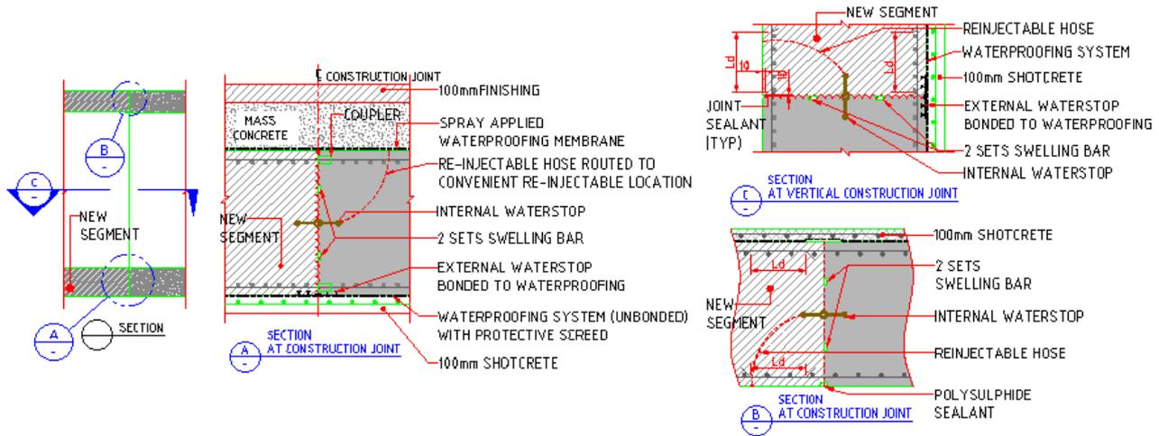
Fig. 4: Construction Joint Details
