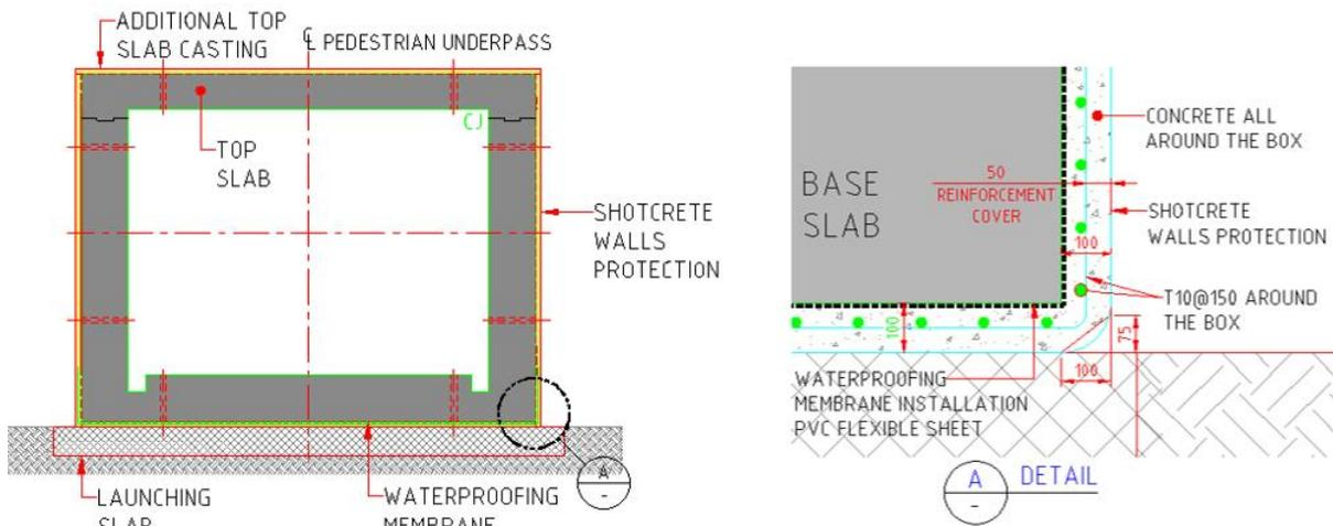
Fig. 3: Waterproofing Membrane Protection
