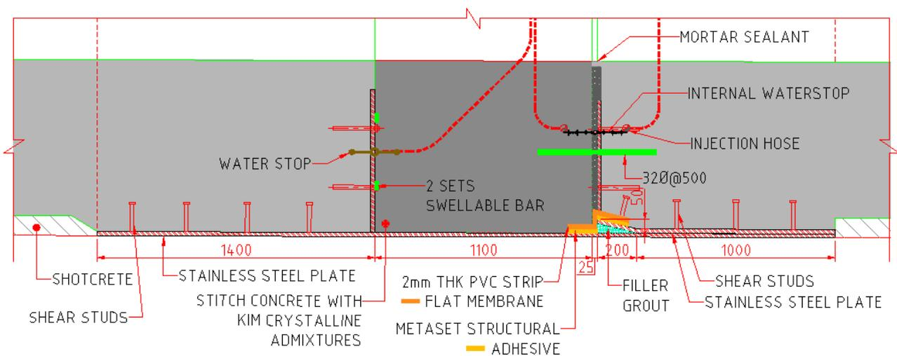
Fig. 5: Expansion Joint Detail at Base Slab
