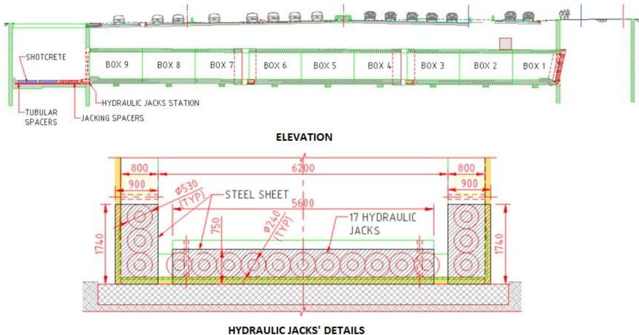
Fig. 6: Box Jacking Arrangement
