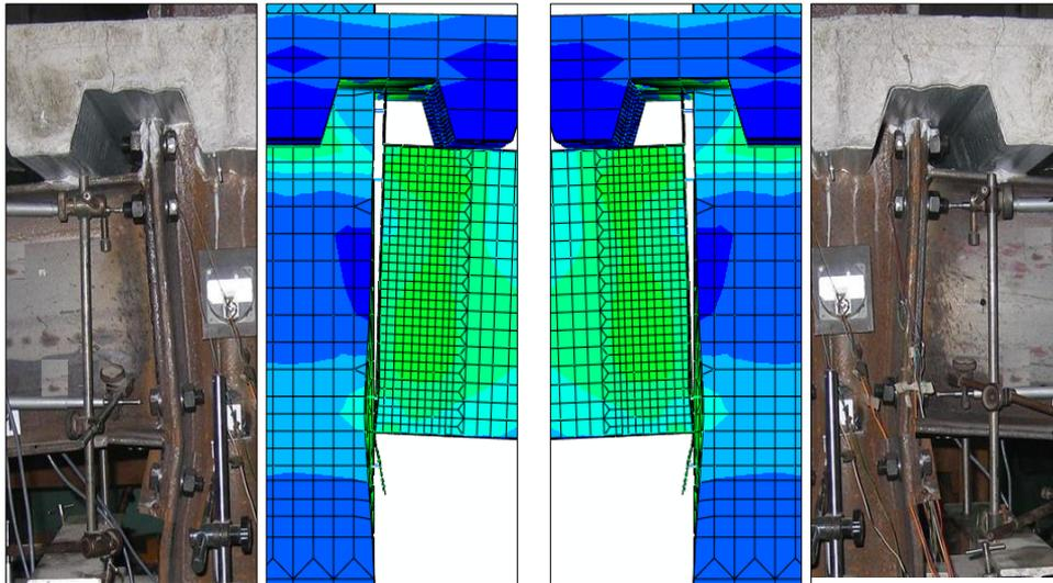
**Fig. 3:** Joint deformation comparison between experimental testing and FEA modelling
