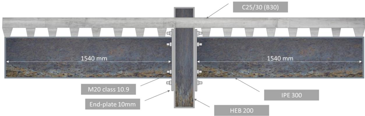
**Fig. 1: Composite symmetric extended end plate joint eight Bolts test (Barcewicz, 2016)**
