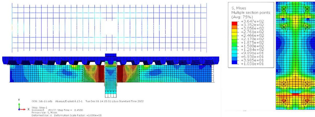
**Fig. 2: Displays the stresses in the joint and the overall model using ABAQUS FE modeling**
