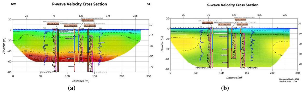
**Fig. 2:** Comparison of the MASW & Refraction data with the borehole controls
