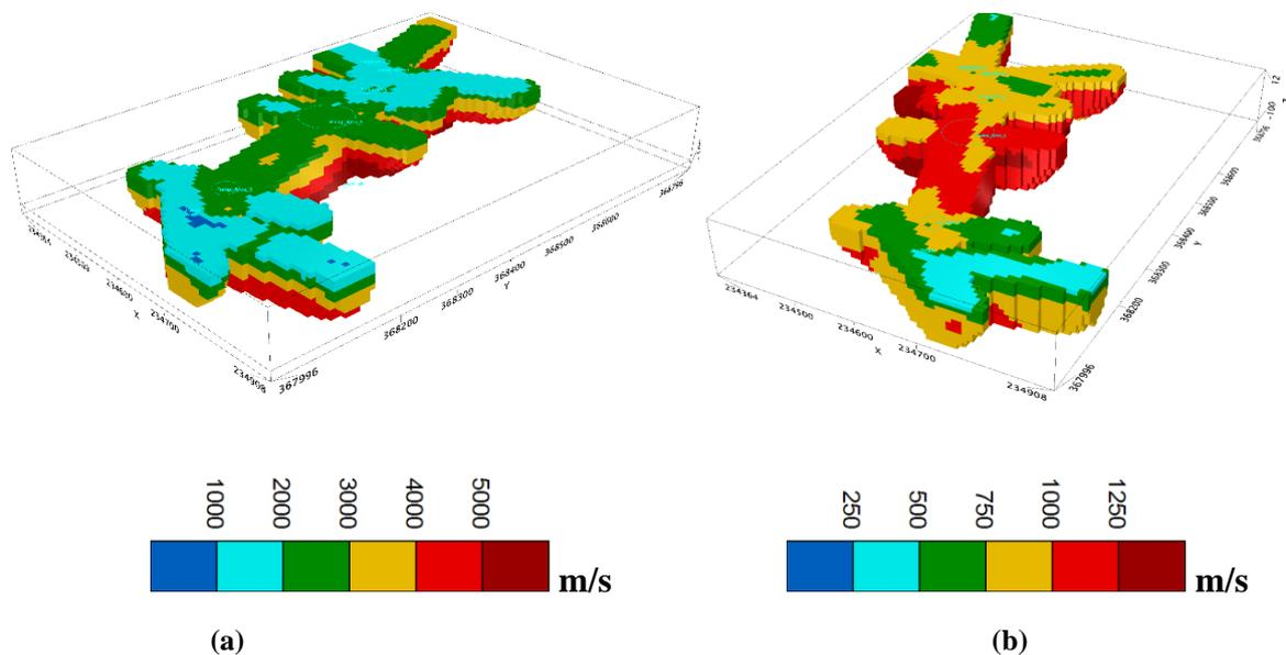
**Fig. 6:** P and S wave 3D Velocity model of one of the critical locations of the project
