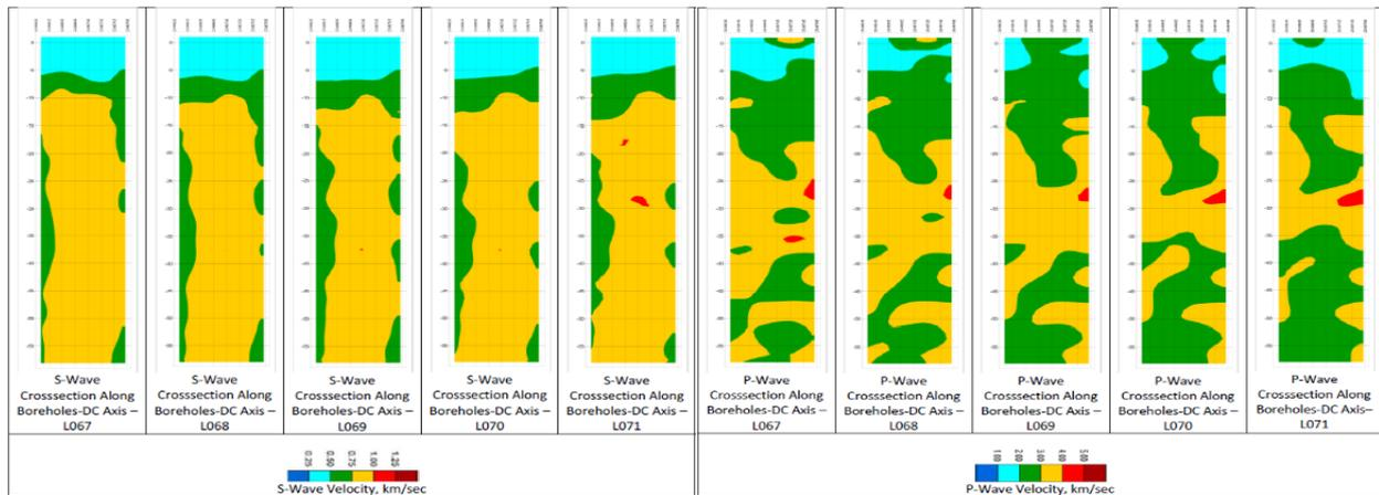
**Fig. 4:** 2D presentation of Results of Seismic Crosshole Tomography
