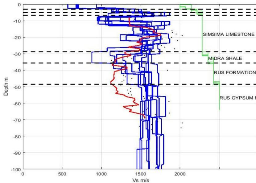
**Fig. 3:** Plot showing the average of all PS-logging values and the geological interpretation (The black dashed lines map the geological transitions onto the geophysical profiles)
