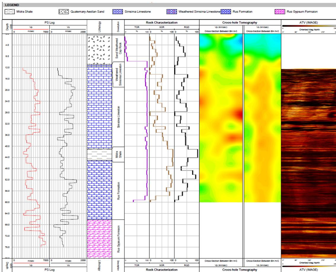
**Fig. 5:** Correlation of Geophysical methods results with the borehole control
