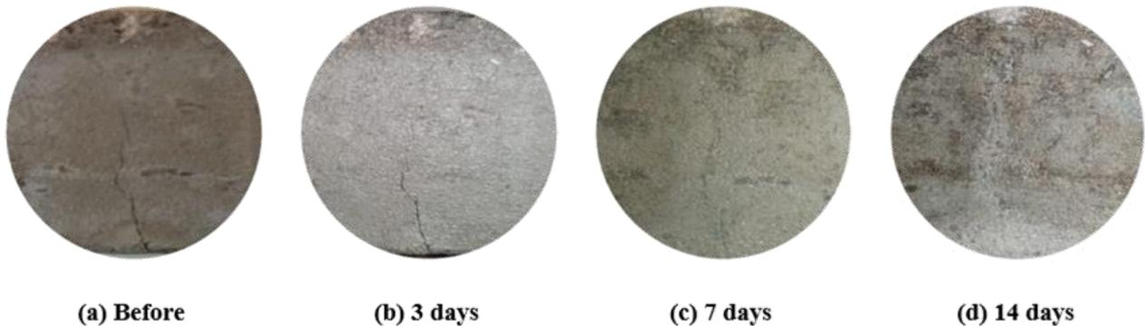
**Figure 6:** Self healing of a Crack Mix C over the Time
