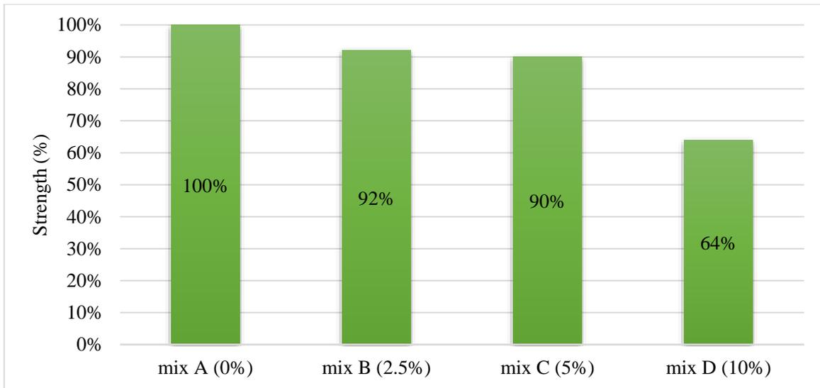
**Fig. 5:** Strength of Different Prisms in Comparison to the Cracking Load of the Reference Mix
