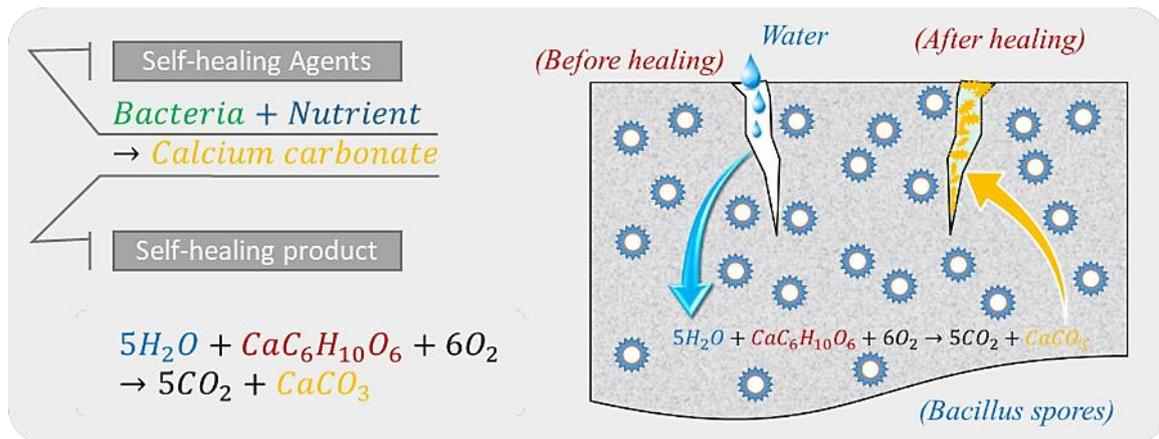
Fig. 1: Mechanism of Self-Healing Concrete
