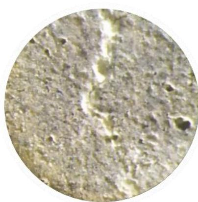
**Fig. 7:** 25x Stereomicroscope Image Showing the Formation of Calcite on a Crack
