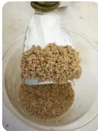
**Fig. 3:** Immobilization of *Bacillus Subtilis* and Calcium Lactate on sand using Gum Arabic
