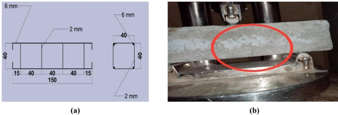
**Fig. 4: Pre-cracking of Mortar Prism**
