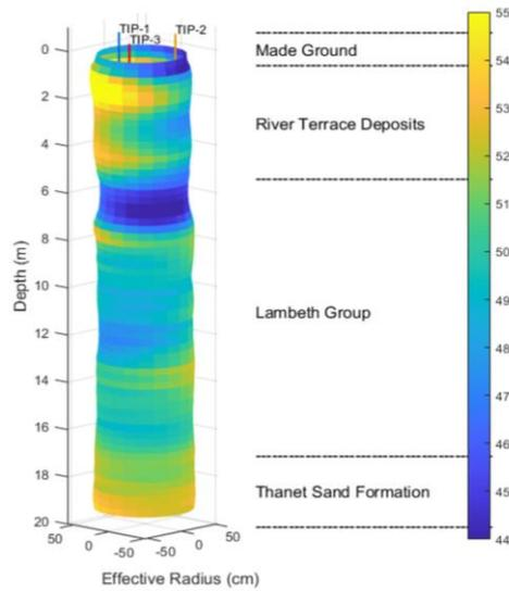
**Fig. 4:** Predicted pile 3D shape
