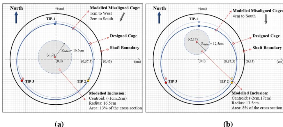
**Fig. 6:** Predicted Anomaly Configurations at (a) 6.1m, (b) 9.4m
