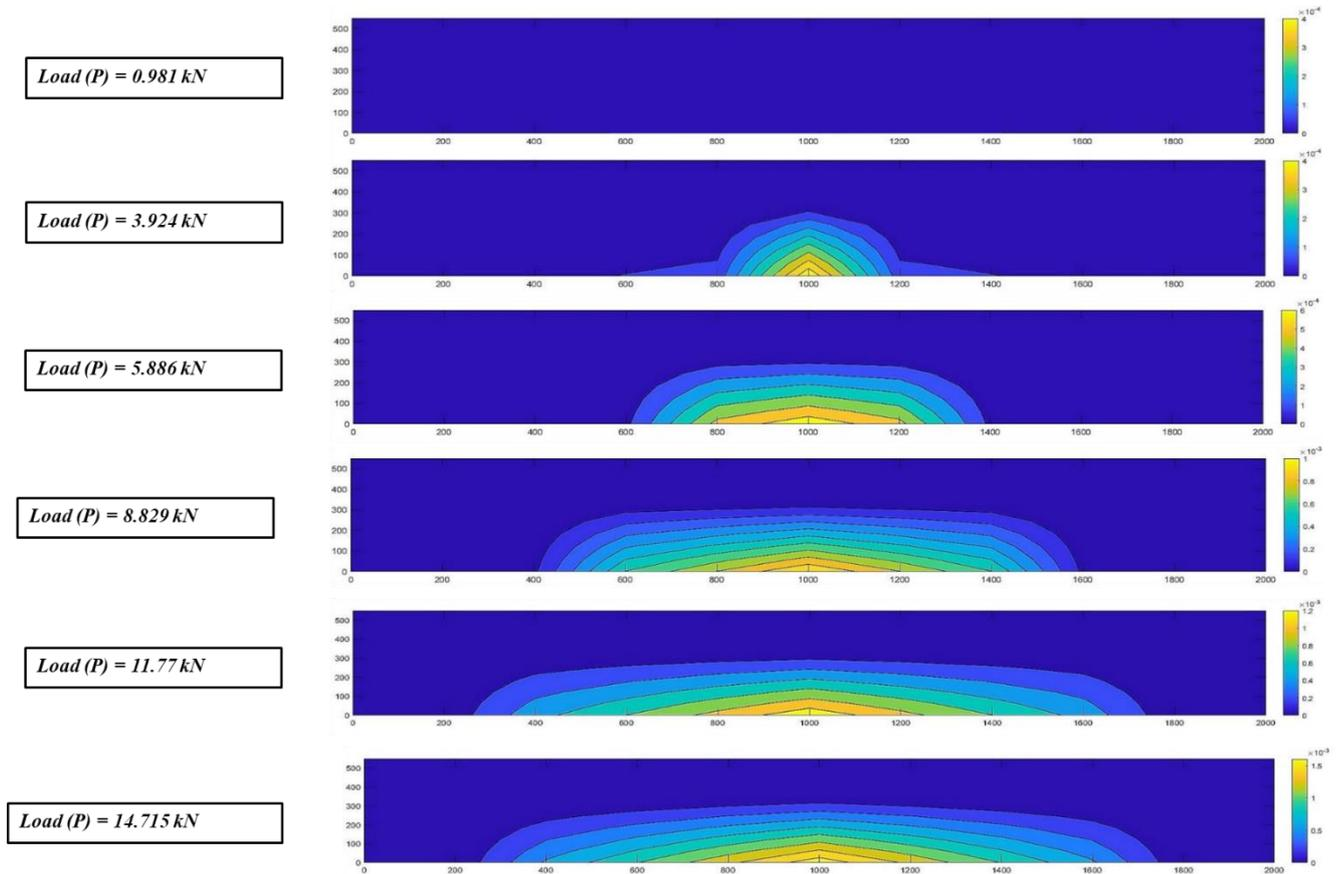
Fig. 2: Simulation of Strain Contour of One-Way Slab
