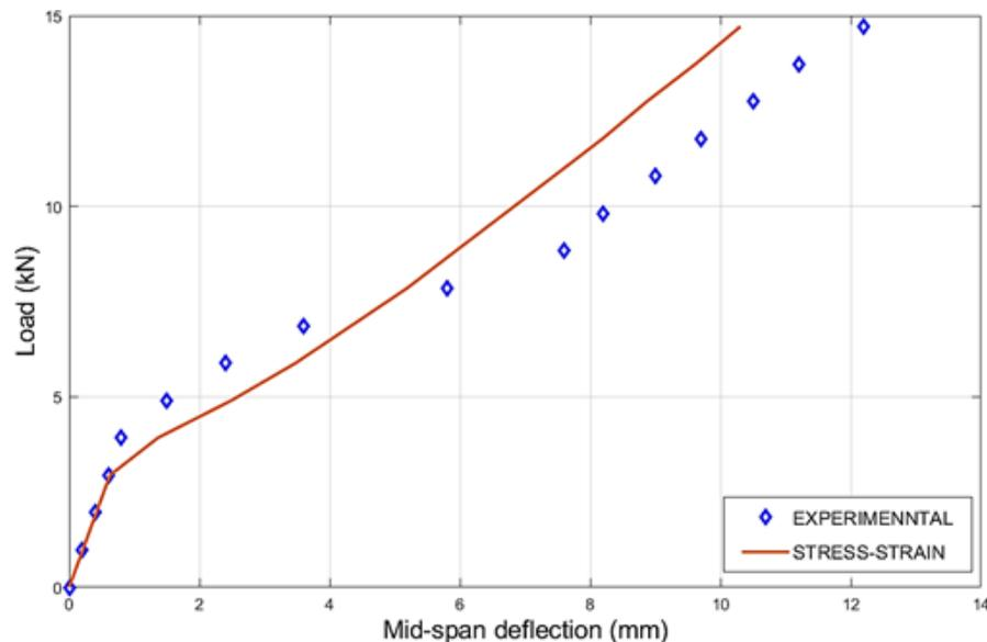
**Fig. 1:** Load-Deflection for a slab subjected to point load
