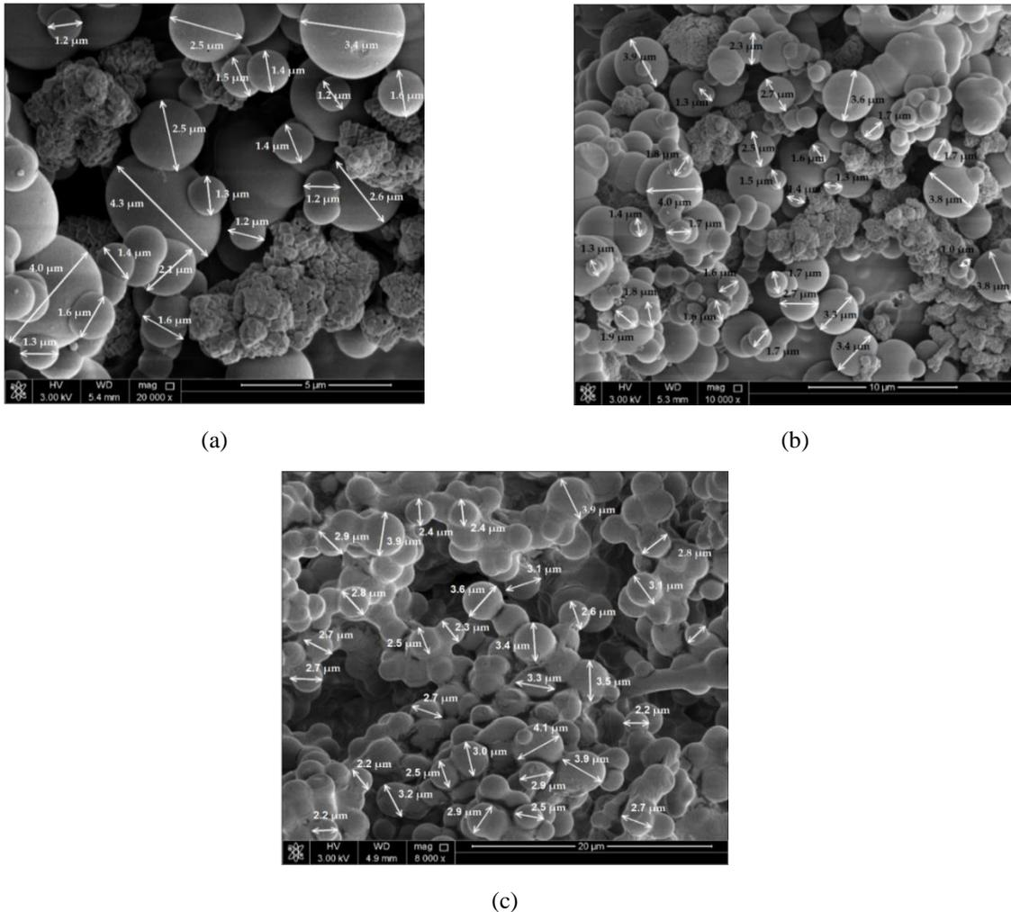
**Fig. 1:** SEM images of the prepared microcapsules showing their diameters at different imaging scales (a)  $5\mu\text{m}$  (b)  $10\mu\text{m}$  (c)  $20\mu\text{m}$
