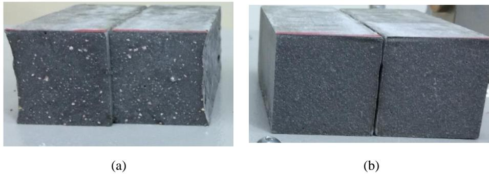
**Fig. 4:** Images of the Prisms' Fracture Surfaces after Flexural Strength Testing (a) Sample Incorporating microcapsules Prepared using the Non-Modified Procedure (without AOT) and (b) Sample Incorporating microcapsules prepared using the Modified Microcapsules (With AOT)
