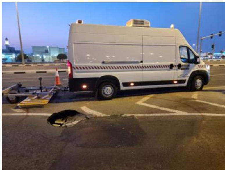
**Fig. 1:** 3D-GPR equipment utilised by Ashghal for Sinkhole investigations
