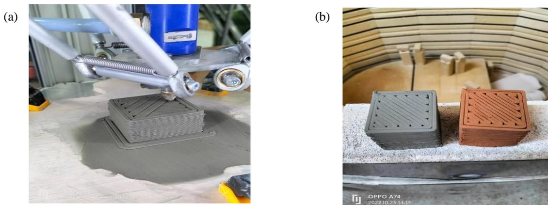
**Fig. 2:** (a) 3D-printing process, and (b) burnt vs unburnt sample
