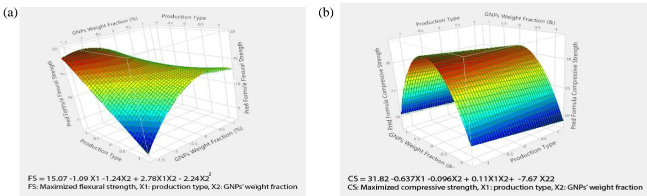
Fig. 4: RSM plots production type and GNPs' weight fraction (a) flexural strength and (b) compressive strength
