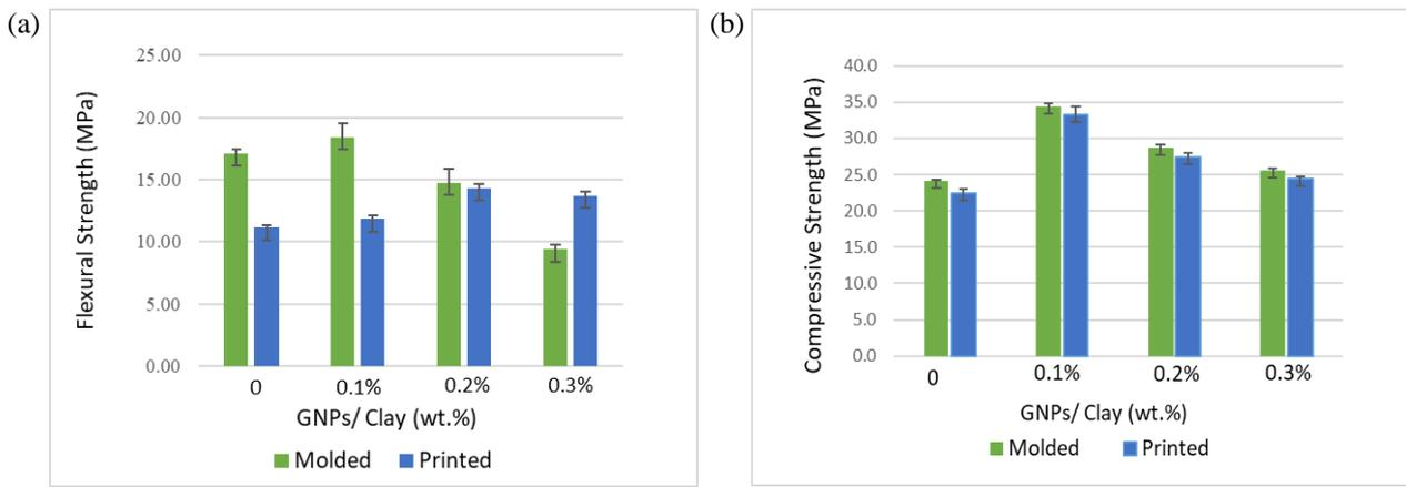
Fig. 3: (a) Flexural strength test results, and (b) Compressive strength test results
