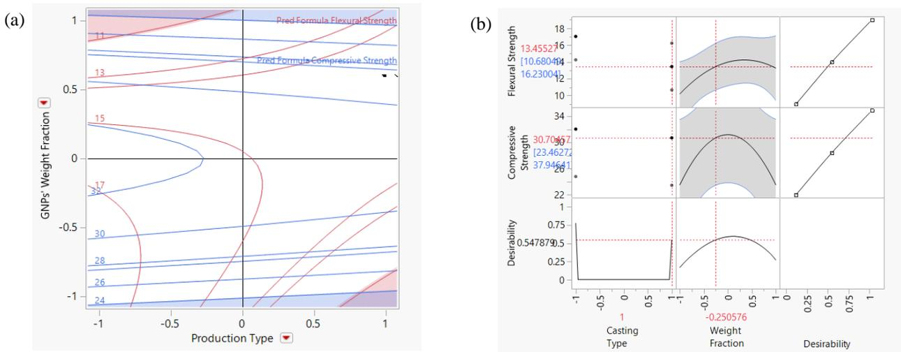
**Fig. 5:** (a) Production type and GNPs' weight fraction variables contour profiles and (b) maximized desirability functions
