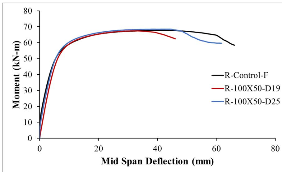
**Fig. 3:** Moment versus midspan deflection curves
