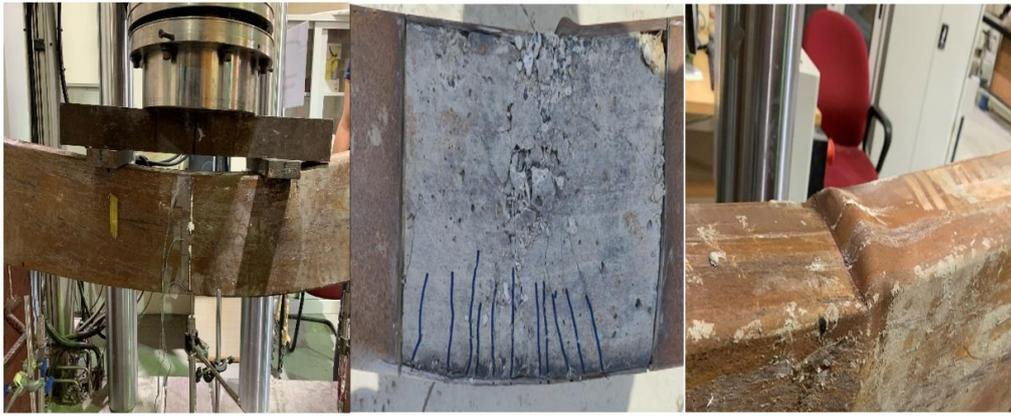
**Fig. 6:** Failure mode of steel and concrete
