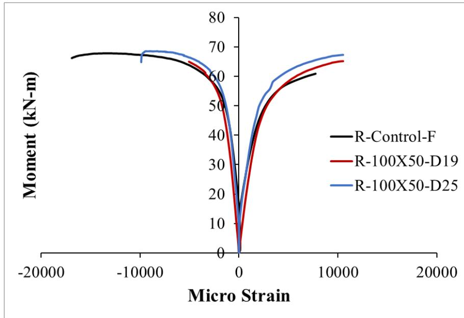
Fig. 4: Moment versus microstrain curves
