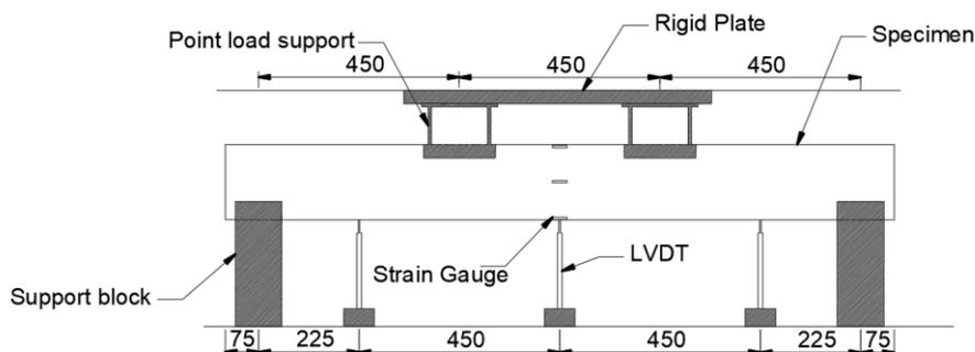
**Fig. 2:** Schematic test setup, dimensions in mm
