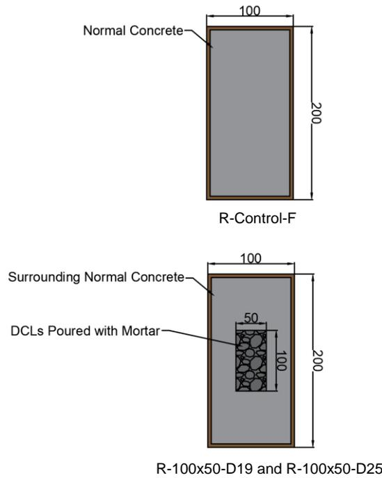
**Fig. 1:** Section details of CFST beam specimens, dimensions in mm
