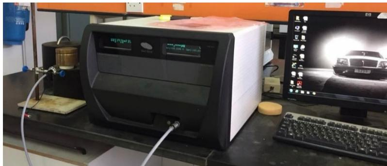
**Fig. 1:** The laboratory arrangement of Hot-Disk 2200 used in this study
