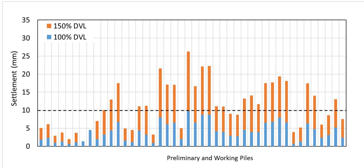
Fig. 5: Settlement of 44 test piles at 100% and 150% of DVL
