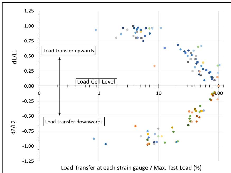
**Fig. 2:** Load distribution along the normalized PTPs length
