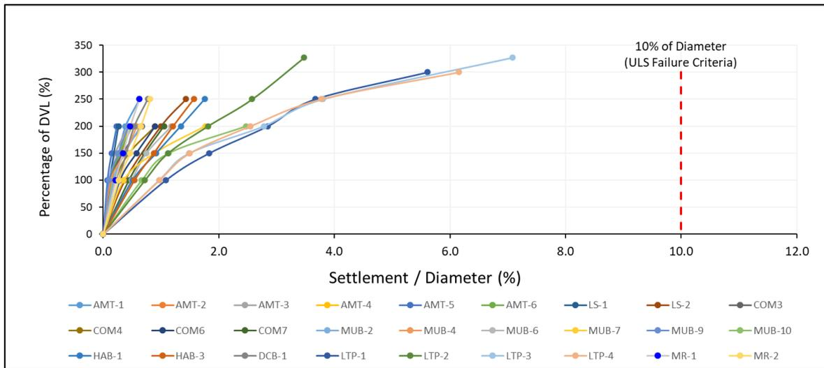
**Fig. 4:** Settlement of trial piles
