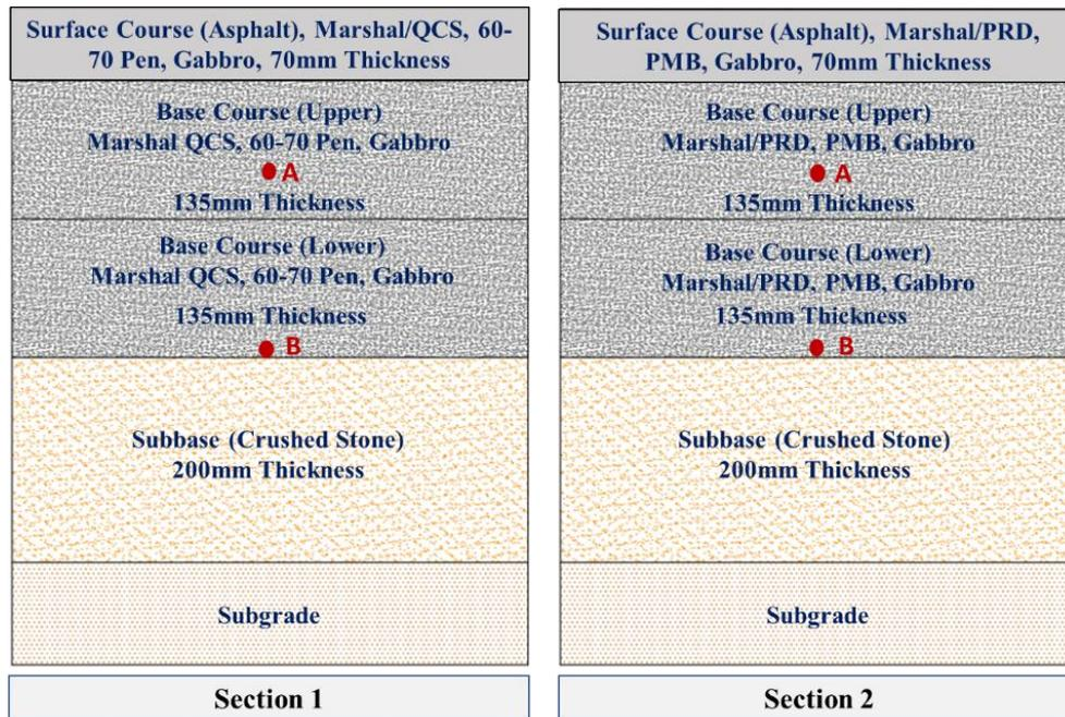
**Fig. 1:** Layers and Materials' properties of the two selected sections
