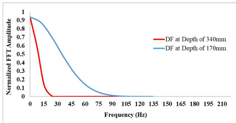
**Fig. 4:** The Frequency domain of loading pulse on section 1 at 72 km/hr during spring
