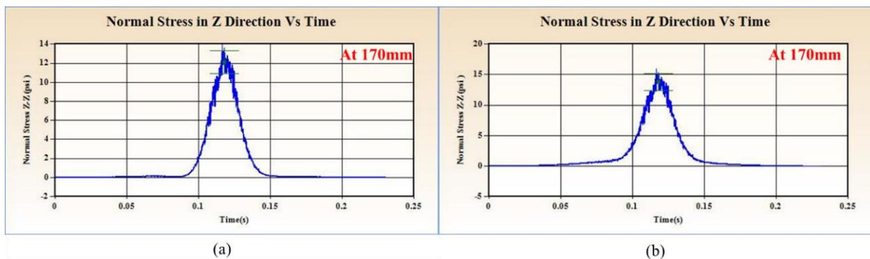
**Fig. 2:** Loading Time Pulse generated on Section 1 at 40 Km/Hr Speed At Depth of 170mm (a) spring season (b) summer season
