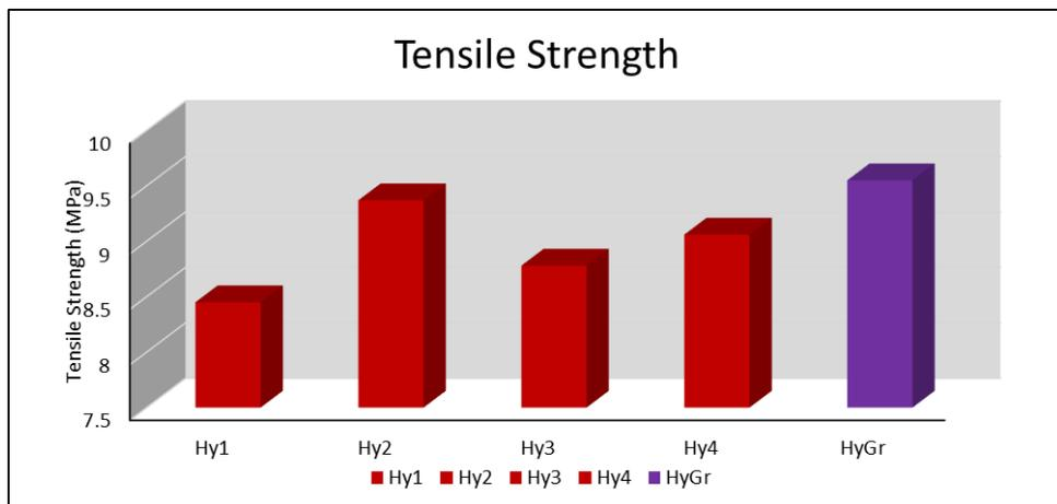
**Fig. 3:** Tensile Strength of HyFR-HSC and HyGrFR-HSC mixes
