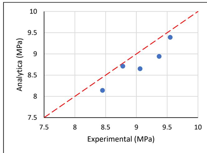
**Fig. 4:** Analytical vs Experimental Composite Tensile Strength of HyFR-HSC & HyGrFR-HSC
