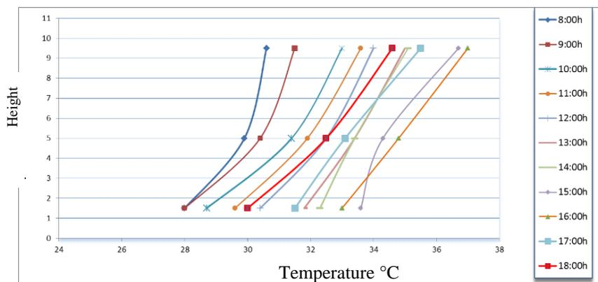
**Fig. 6:** The vertical thermal profiles of air temperatures recorded in center of the atrium for different hours of the day
