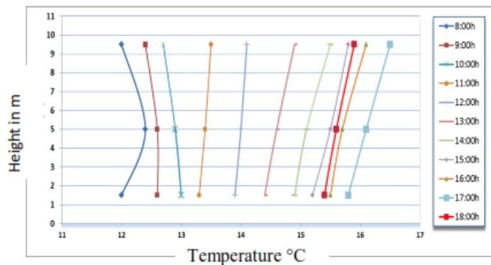
**Fig. 8:** The vertical thermal profiles of air temperatures recorded in center of the atrium for different hours of the day
