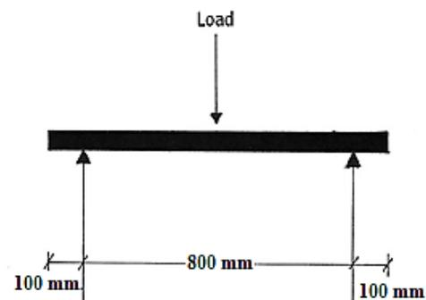
**Fig. 2:** Loading set up for the experimental work
