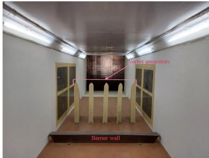
**Fig. 1:** Upstream Portion of the Test Section of the Wind Tunnel
