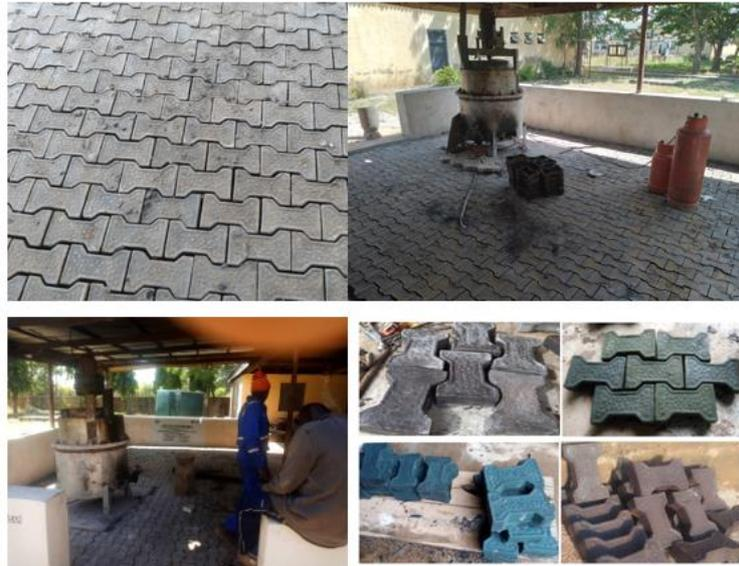
**Fig. 5:** Densifier Machine and Various Colors of Plastic-Laterite Interlock Bricks
