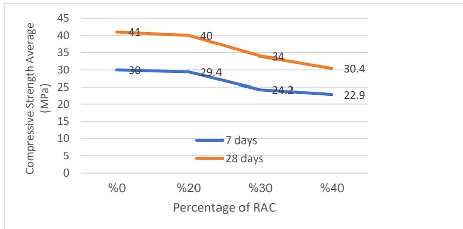
**Fig. 3: Compressive Strength Results for 7 & 28 days****Table 2: Compressive Strength Results**
