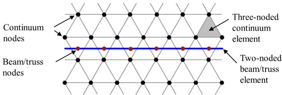
Fig. 3: Concept of the constraint nodes
