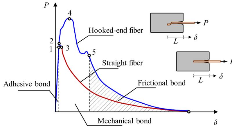
Fig. 1: Schematic representation of pull-out load-slip behavior, adapted from Kooiman (2000)
