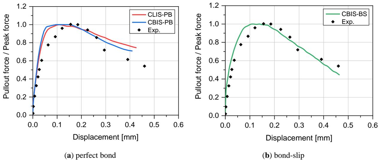
Fig. 6: Pull-out-displacement curve in comparison to the simulation results
