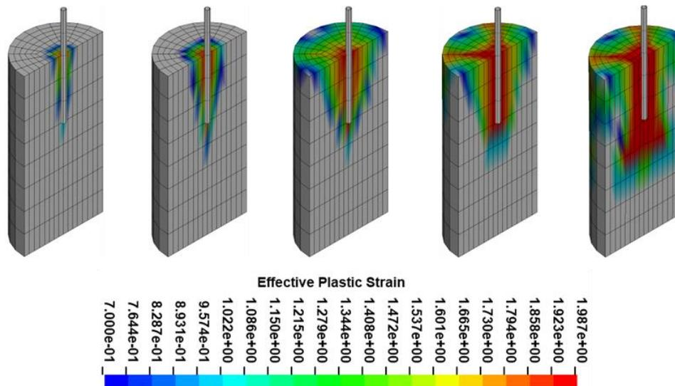
Fig. 7: Damage states at the center cut plane for the CBIS-PB configuration
