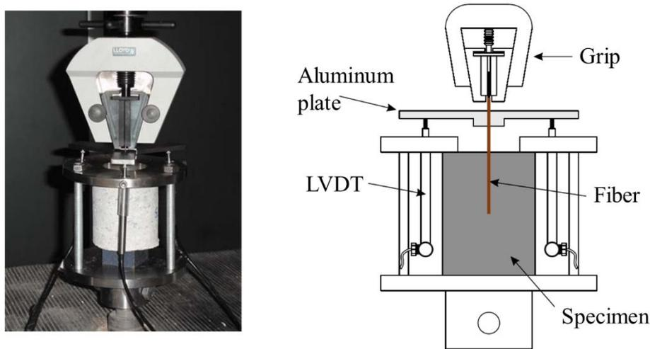
**Fig. 4:** Single fiber pull-out test setup, according to Shannag et al. (1997)
