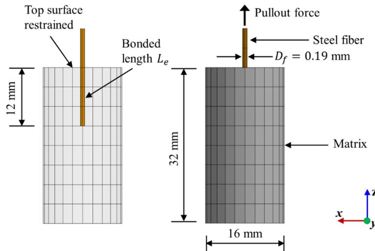
**Fig. 5:** Finite element discretization of single fiber Pull-out test
