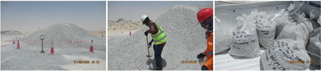
**Fig. 2:** RCA material stockpile and sampling at QPMC
