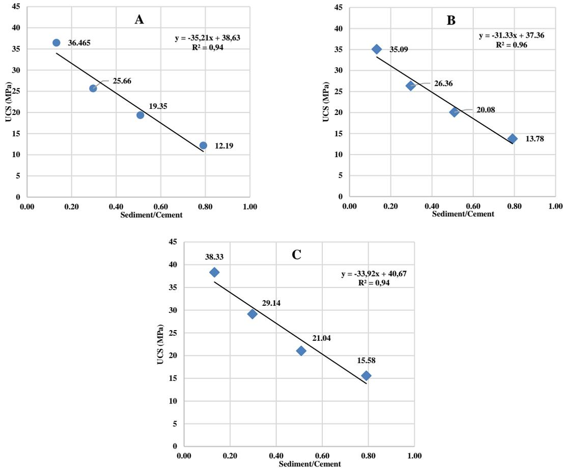
**Fig. 1:** Mix mechanical strength versus S/C ratios (A: Cement CEM I 52.5 N, B: Cement ROLAC PI LH, C: Cement CEM I 52.5 PM ES)
