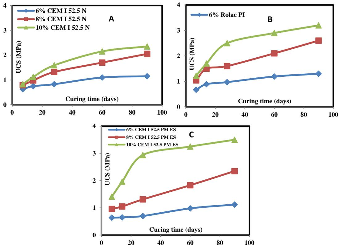
**Fig. 2:** Compressive strength of various prepared mixes (A: Cement CEM I 52.5 N, B: Cement ROLAC PI LH, C:
