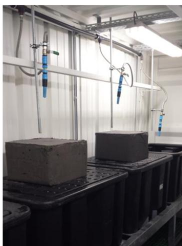
Fig. 3: Grout block leaching test
