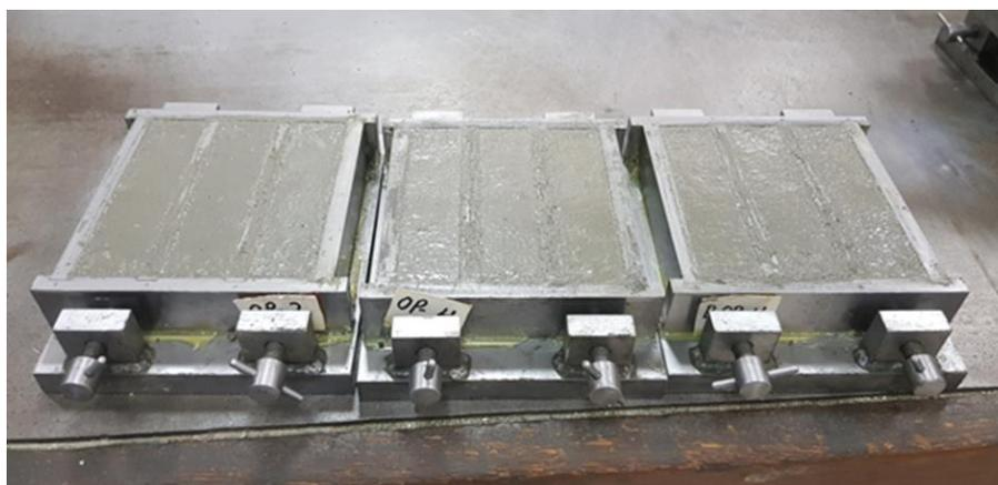
**Fig. 3:** Casting of the fresh mortar prisms
