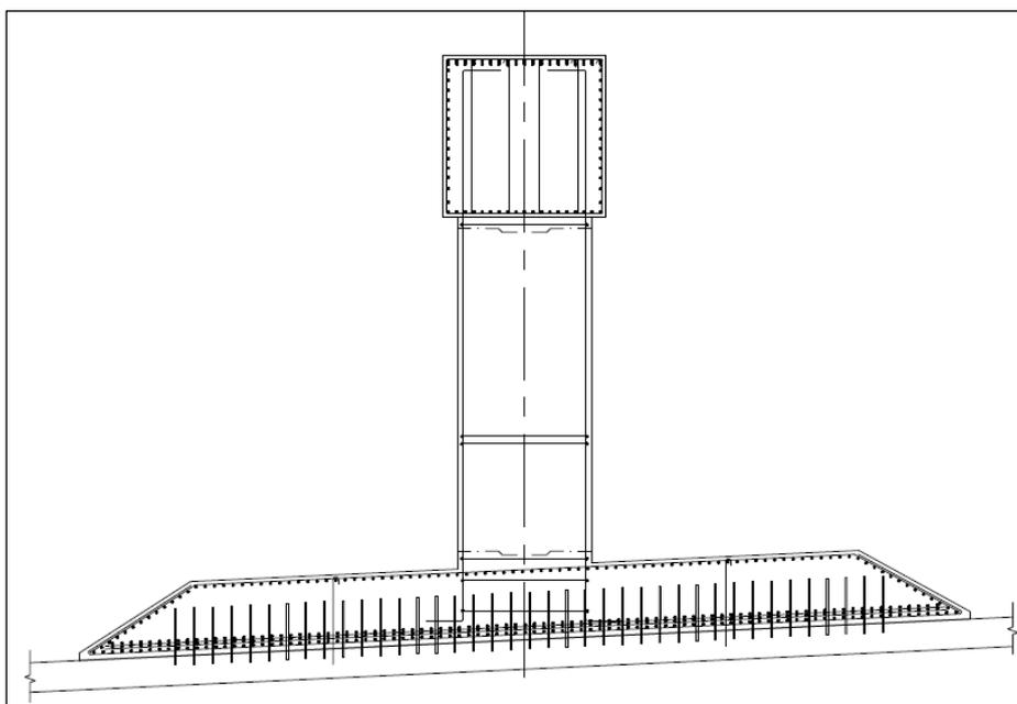
**Fig. 8:** Median Pier integrated footing
