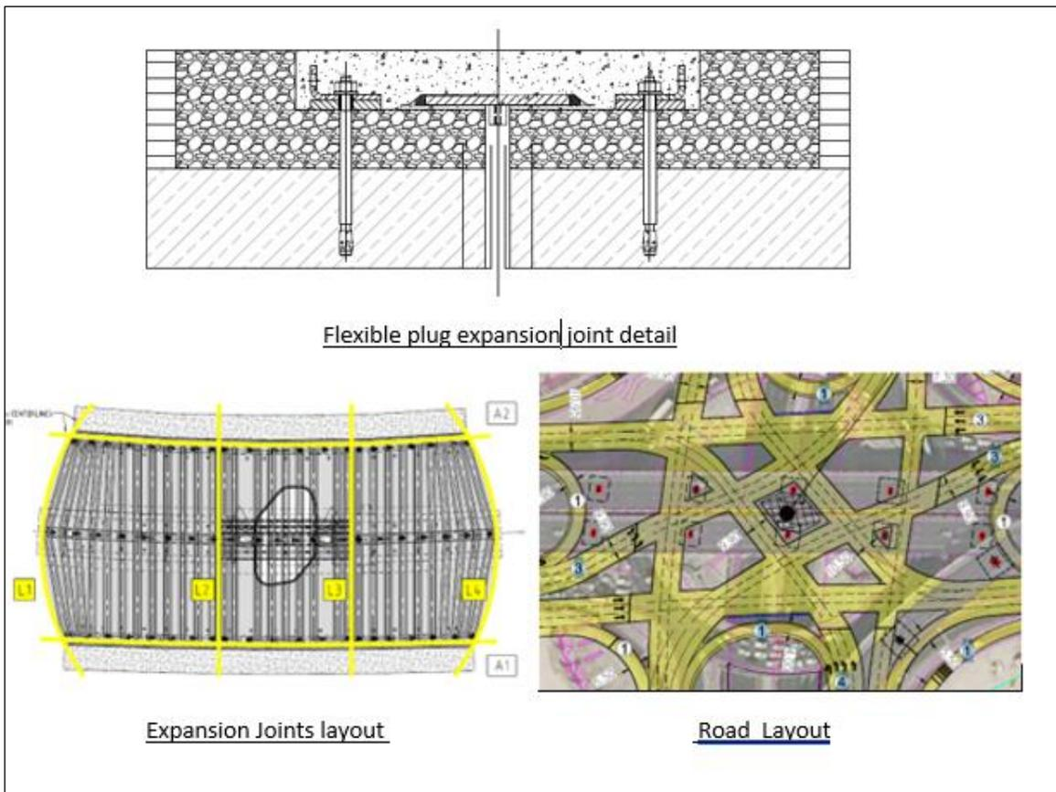
**Fig. 7:** Flexible plug expansion joints details and layout
