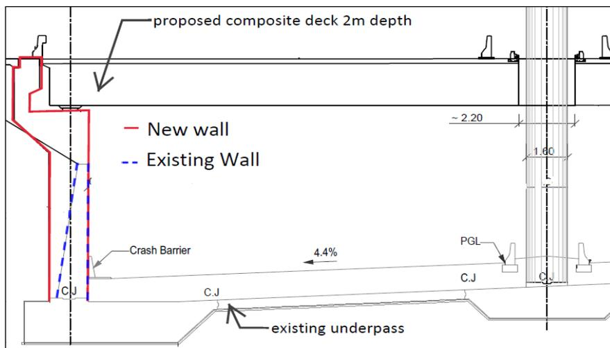
**Fig. 2:** Reference Design Typical Section
